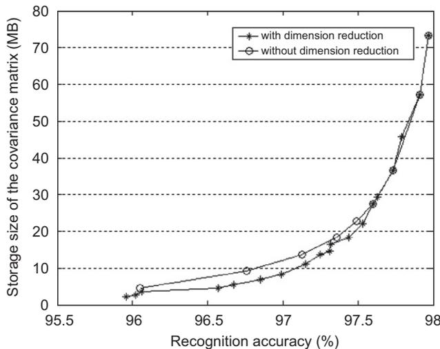
Fig. 6. The tradeoff curves with dimension reduction by choosing different  $D_L$  and without dimension reduction for eigenvectors.
