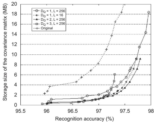
Fig. 8. The tradeoff curves of by choosing different  $D_Q$  and  $L$ .
