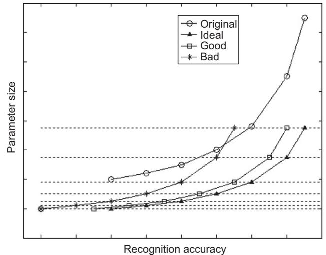
Fig. 4. A hypothesis of tradeoff curves between parameter size and recognition accuracy.
