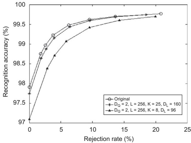
Fig. 9. The error–reject tradeoff curves of the original and compact MQDF classifier.
