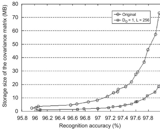
Fig. 7. The tradeoff curves of the original parameters and the compressed parameters by  $D_Q = 1$ ,  $L = 256$ .
