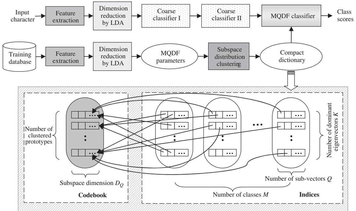
Fig. 3. Block diagram of the recognition system using the compact MQDF classifier.
