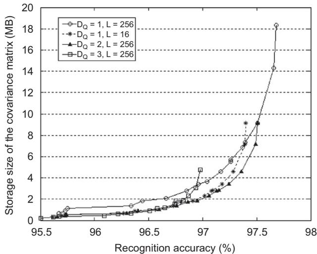
Fig. 10. The tradeoff curves of by choosing different  $D_Q$  and  $L$  based on the cleaned-up database.
